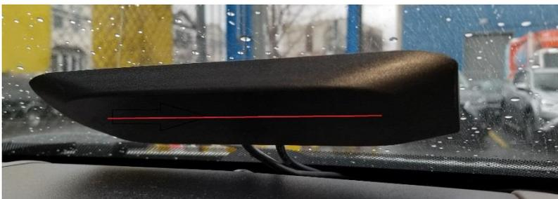
Fig 3. Bottom Side Windshield Mount Antenna (Interior View)
