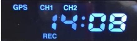
4. Allow Recorder to run for a few minutes. Turn the vehicle ignition off and confirm the LCD display dims/blinks slowly, indicating Parking Surveillance Mode. Refer to [p.19](#) to safely remove the SD card.
