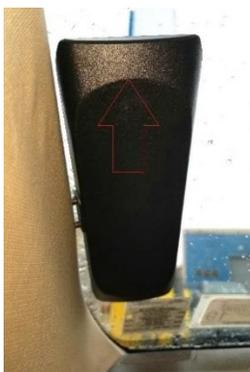
Fig 1. Left Side Windshield Mount Antenna (Interior View)
