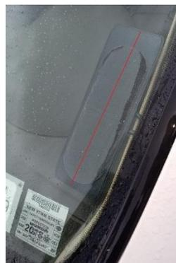
Fig 2. Left Side Windshield Mount Antenna (Outside View)
